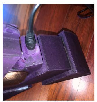
Figure 3-2 DC Barrel Jack Holder Installed
