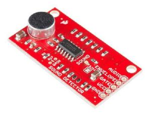
Figure 7-3 SparkFun Sound Detector
