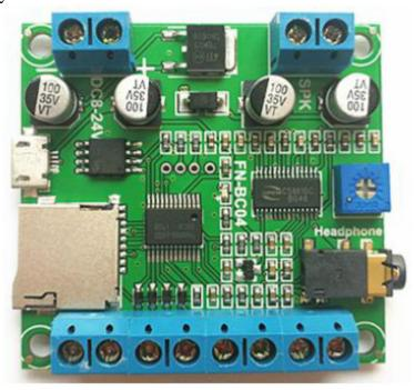
Figure 7-1 Electronics123.com, Inc. 4 Buttons Triggered MP3 Player Board
